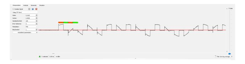
I marked the signal here with red and green. Red is where the signal is present and green where no signal is present. This looks pretty much like OOK (On-Off Keying), where a high amplitude is used to represent a binary 1 and the absence of any amplitude to represent a 0. The morse signal is a well known example of OOK.
