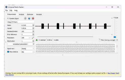
The Autodetect thinks the signals are 200 Samples/Symbol, but this is not correct. When switching the Signal view to "demodulated" we can actually have a better look and measure the correct value there.
