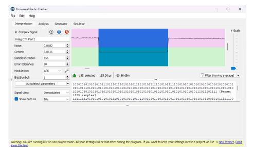
With the values for the Samples/Symbol now to 155 and an errorrate of 20 we can switch now to the Analysis tab.
